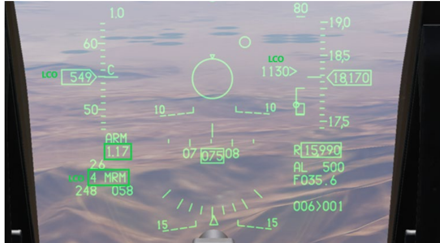
Figure 16: Mockup of the Predictive Feedback display in the HUD using a screenshot of the HUD in DCS. LCO markers are present next to the missile selected, airspeed, and DLZ Caret. Flashing boxes are drawn around the Mach and weapon selected.
