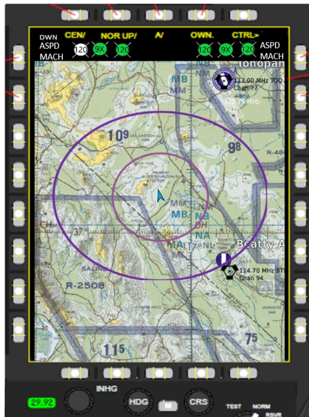
Figure 4: The Predictive Feedback display at the top of the CDU TAD page, with the moving map and range rings. The left Airspeed (ASPD) and Mach are the download envelope limits (DWN) and the right values are for the current envelope. The currently selected missile is shown in white. The labels for the CDU Option Select Buttons (OSBs) were not shown because the buttons were not functional.
